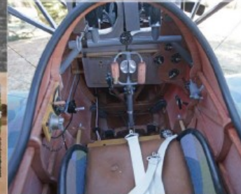
Karl's Albatros - 1/4 scale, functional control stick and rudder bar, water cooled engine, two machine guns, functional lever-operated louvers on watercooler in upper wing
