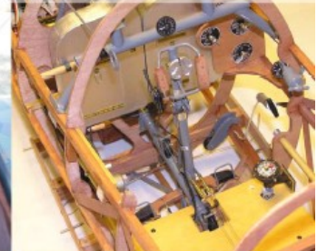
Karl's Albatros - 1/4 scale, functional control stick and rudder bar, water cooled engine, two machine guns, functional lever-operated louvers on watercooler in upper wing
