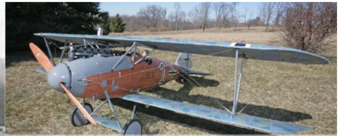
Karl's Albatros - 1/4 scale, functional control stick and rudder bar, water cooled engine, two machine guns, functional lever-operated louvers on watercooler in upper wing
