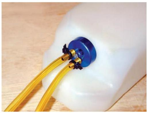
Even when using gasoline-grade fuel tank hardware and fuel lines (Sullivan Products shown here), be sure to secure the fuel line inside and out with some clamps or cable ties, as shown here.
