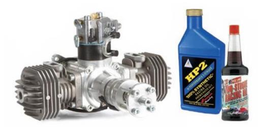
Regardless of the fuel-to-oil mixture ratio you use, it is important to use good-quality oil. Cheap oil can risk the health of your engine. The 40cc RCGF 40T engine is shown at the lower left.
