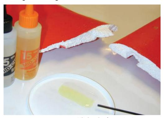
**Step 1:** In extreme cases, you might break a foam wing in two (or more!) pieces. A great trait of foam is that it is usually very easy to piece back together. Mix up a small batch of 15-minute epoxy on a plastic can lid. Run two or three lengths of each part as shown and then mix together.
