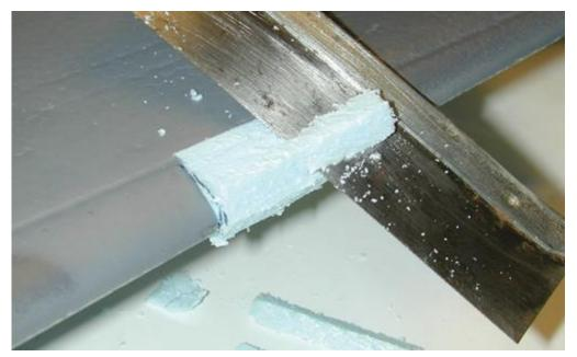
**Step 3:** Cut some new foam to length, and glue it in place with foam-safe CA. The best way to do this is to cut the foam a bit oversize, and spray foam-safe accelerator to the new material. Apply the CA glue to the cutout area, and insert the repair piece. Hold it in place until the glue sets. Use your saw to remove most of the unwanted material, then use a sanding block to smooth the replacement piece.
