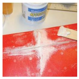
**Step 5:** After the glue sets, apply model filler to the repair and let the filler dry.
