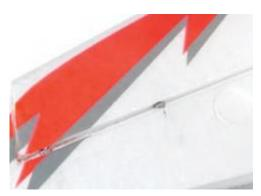
**Step 6:** Apply more glue inside the holes in the vertical fin, and slide the hinges in the rudder into place. Again, wipe away any adhesive that oozes out of the holes with paper towels and alcohol. Set aside until the epoxy sets.
