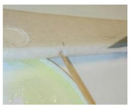
**Step 4:** Mix up some 15-minute epoxy, and use a toothpick to apply the adhesive into each of the holes in the rudder.
