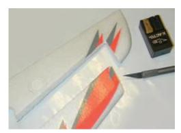
**Step 2:** After marking the hinge locations, take a sharp hobby knife and slice through the molded hinge to separate the rudder from the fin. Use some sandpaper to smooth the mating surfaces.
