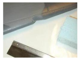
**Step 1:** The leading edge of a foam wing can really take a beating, but dents are really only cosmetic issues. If you have a minor dent, simply apply a wet paper towel to it and heat with a covering iron. Most of the time, the steam will expand the foam and your dent will disappear.
