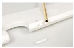
**Step 3:** Sharpen the end of a 1/8-inch brass tube, and use it as a drill to produce the holes for the Hinge Points. This produces much neater holes than a wood drill bit.
